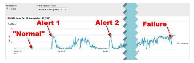
Above is a chart of Simularity's Predictive Failure Signature for the sensor data preceding the failure. After a period of normal operations, two significant alerts appear 45 and 33 days in advance of the failure. Had the customer known beforehand that this failure was looming (Alert 2), things would have been different:
