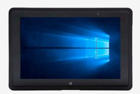
The Windows-based aegex10 Intrinsically Safe Tablet is certified for use in ATEX/IECEx Zone 1 and Class I Division 1 hazardous areas of industrial operations where combustible materials are present, including drilling platforms.
